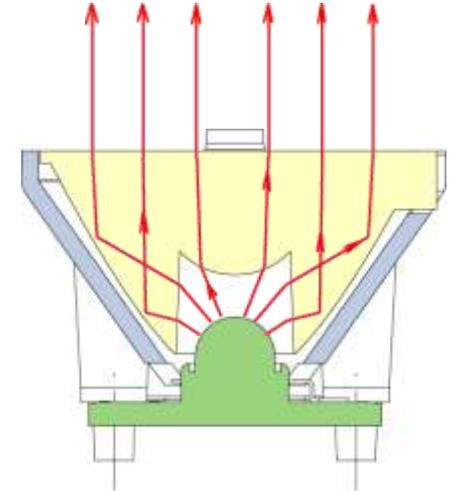
**Picture showing Carclo 20mm diameter frosted optics**
